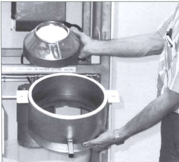
The fruit moves over the grater before the juice passes thru the screen and into the juice collector.
