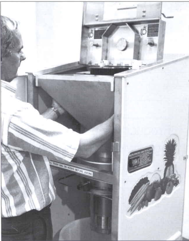
The hopper lifts out for easy cleaning and re-assembly, 1 of 5 removable parts.
